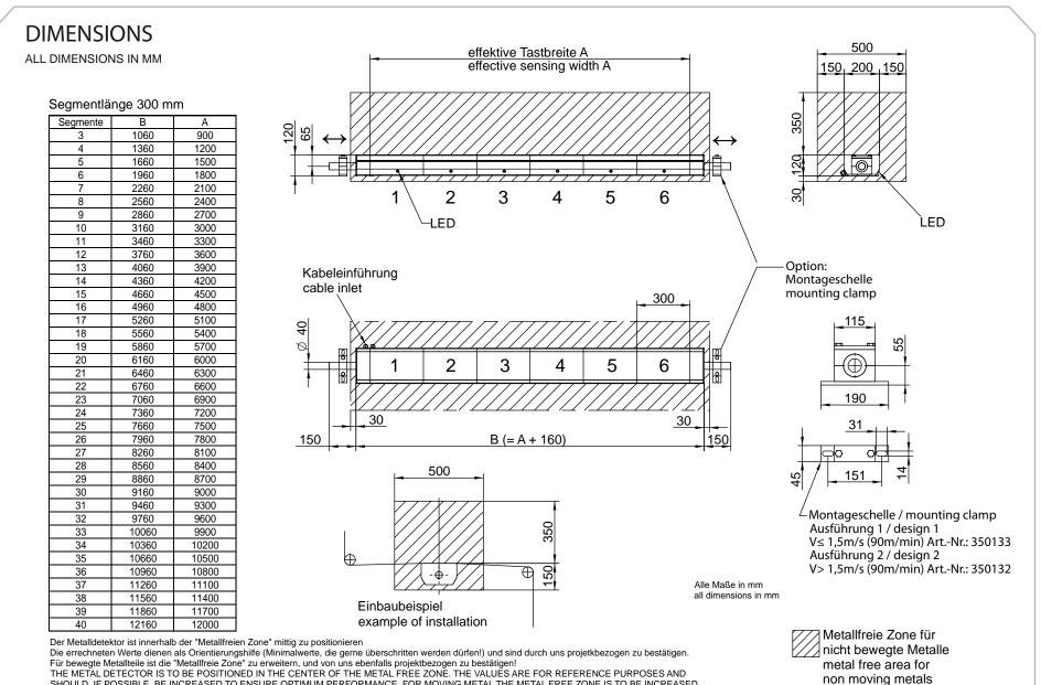
SHOULD, IF POSSIBLE, BE INCREASED TO ENSURE OPTIMUM PERFORMANCE, FOR MOVING METAL THE METAL FREE ZONE IS TO BE INCREASED AND TO BE CONFIRMED BY A REPRESENTATIVE.
