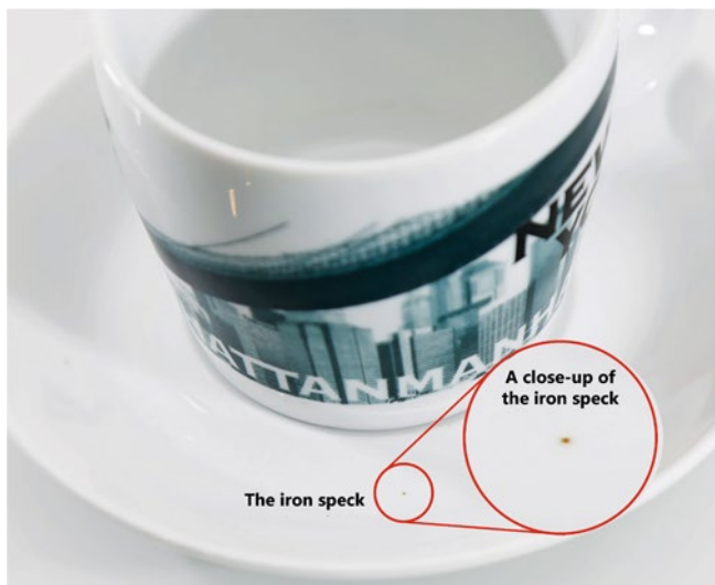
Figure 1 Iron speck contamination in fired ceramic tableware (© Paul Fears Photography)
