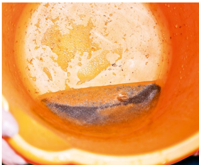
Figure 3 Paramagnetic minerals separated using an electromagnetic filter (© Paul Fears Photography)
