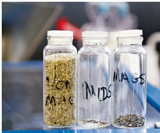
Figure 2 Three fractions after magnetic separation – non-magnetics, middlings and magnetics (© Paul Fears Photography)
