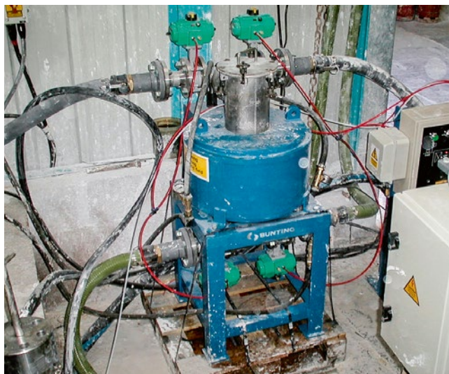
Figure 4 Bunting electromagnetic filter in a ceramics plant (© Bunting)
