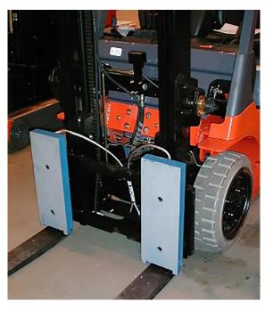
Forklift Stabilising Magnets are designed to retain sheet steel loads, holding them against the forks during lifting or transportation.
