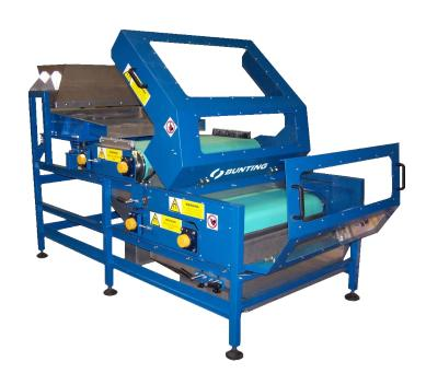
The Bunting Rare Earth Roll incorporates Neodymium Iron Boron permanent magnets, which are the most powerful magnets available and are built into a composite high-intensity magnetic head pulley.
