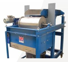
Typical applications of Permanent Drums include the separation of steel swarf from aluminium and for the removal of ferrous contaminants from shredded wood and glass cullet.
