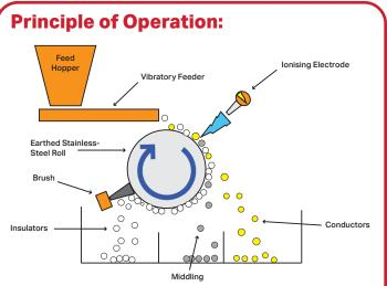
Material is fed onto the revolving stainless-steel earthed roll (typically 20-50 rpm) and subjected to a high- tension discharge from a fine tungsten wire electrode. Poor conductors (insulators) remain charged, are pinned by an image force on the roll surface, and then are discharged by the brush. Conductors quickly lose their charge and are thrown off the roll on their natural trajectory.
