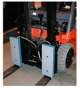
Forklift Stabilising Magnets are designed to retain sheet steel loads, holding them against the forks during lifting or transportation.
