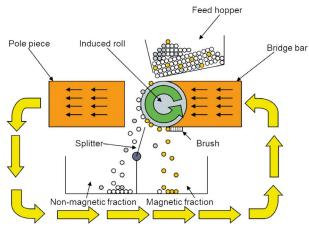
Principle of operation of Induced Roll Separator
