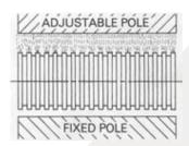
The roll design and electro coil design gives an infinitely variable field strength up to 2 Tesla on the roll surface allowing the efficient separation of weakly paramagnetic minerals.
