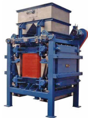
Induced Roll Separator: 1 metre width, 2 pass unit used for processing nepheline syenite.
