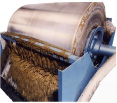
The Wet Drum Magnetic Separator features a strong, stationery permanent magnetic element mounted inside a revolving non-magnetic shell. The adjustable multi-pole ceramic ferrite magnetic element produces a high-flux, radial magnetic field (along the circumference of the shell), which maximises recovery to + 99.9%
